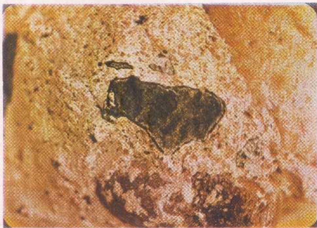
Fig 3 Dark reaction rims on aggregate
