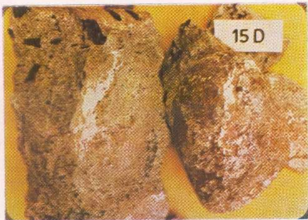
Fig 2 Gel formation on the aggregate
