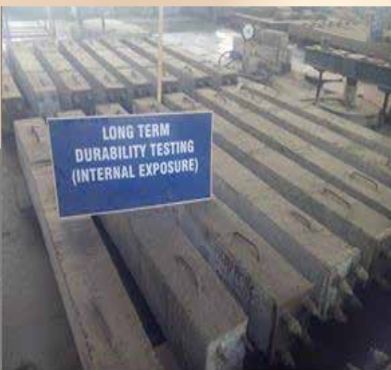
Long Term Durability Studies on Pre-stressed Concrete Beams
