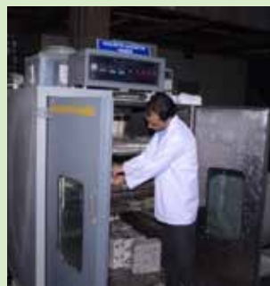
Accelerated Carbonation Studies as per ISO 1920:Part-12
