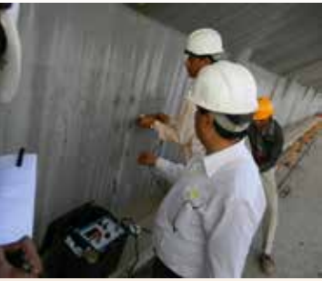
UPV Test of Concrete Structure for Quality Assessment
