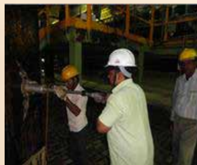
Core Extraction from Fire Damaged Structure
