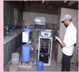
Under Water Abrasion Testing as per ASTM C1138
