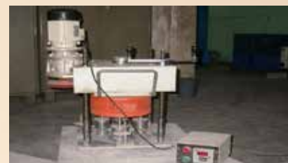
Abrasion Resistance Test for Concrete
