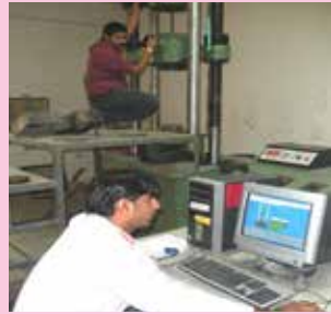
5000 KN UTM Machine for testing of Reinforcing Steel
