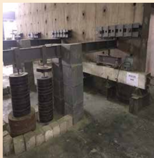
Long Term Creep Testing on Pre-stressed Concrete Beams (In Flexure)
