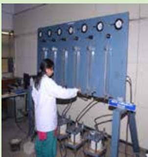
Water Permeability Testing as per DIN 1048 Part-5
