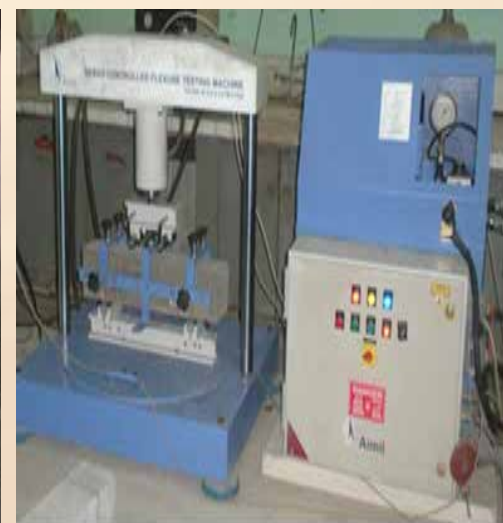
Flexure Toughness Test on Steel Fibre Reinforced Concrete
