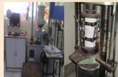
Confined & Unconfined Compressive Strength Determination for Plastic Concrete
