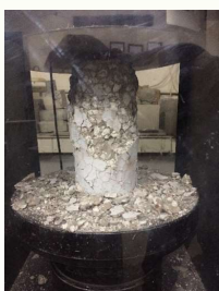
(a) Sample under testing after fire exposure
