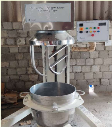
Planetary mixer developed at NCB for preparation of UHPC
