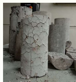
(b) Sample texture after fire exposure
