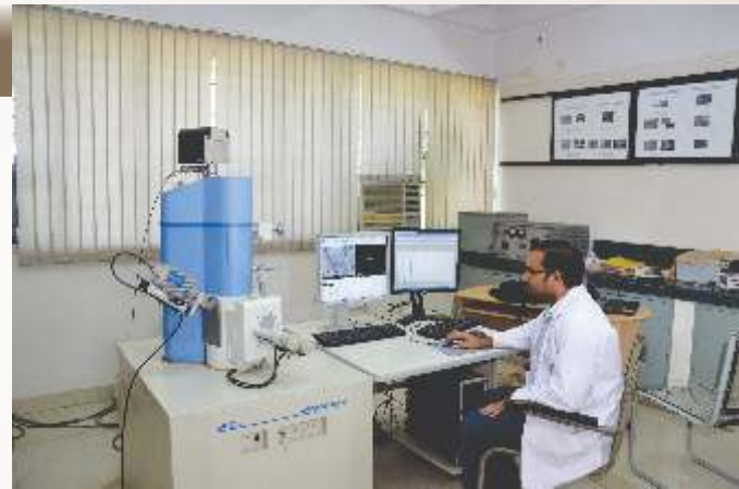
Scanning Electron Microscope with EDAX for morphological and microstructural studies of cement, concrete etc
