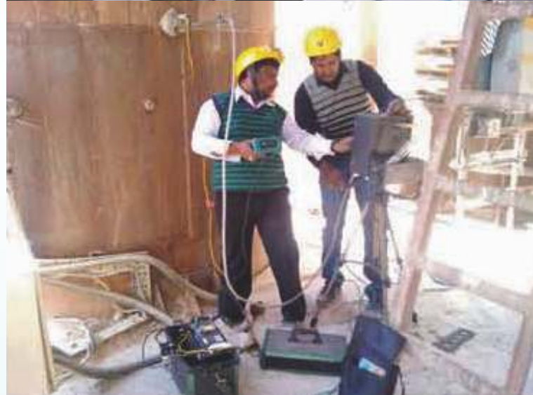
Monitoring of PM & Gaseous Emissions at Kiln Stack
