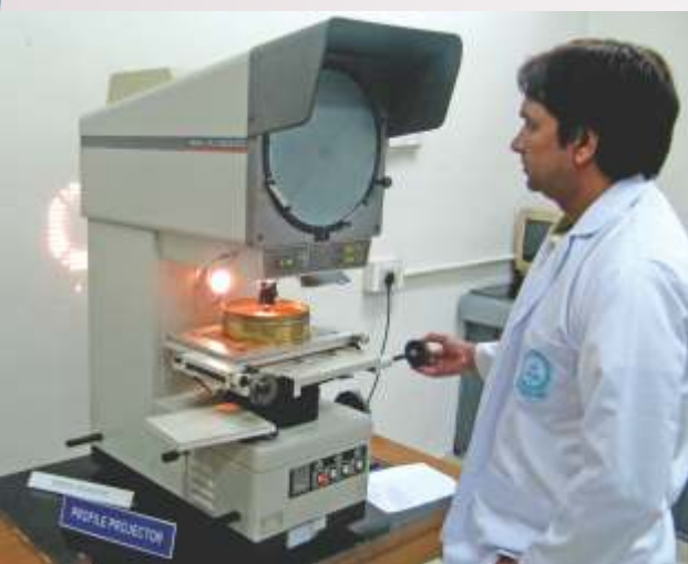
Calibration of Sieve at Profile Projector
