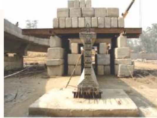
Load Test on Pretension Girder for Flyover Project
