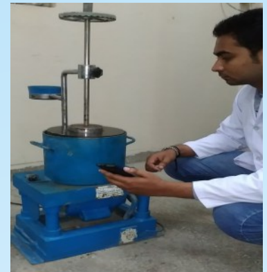
Workability Measurement of Roller Compacted Concrete
