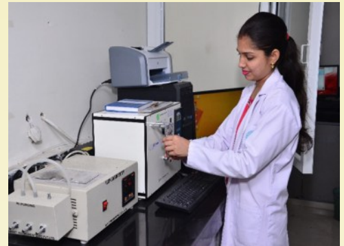
BET Apparatus for determining fineness of ultra-fine powder materials such as silica fume, metakoline, ultrafine fly ash, ultrafine slag etc.
