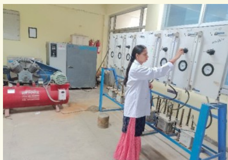
Water Permeability Test on concrete samples.
