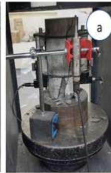
Failure mode of tested concrete specimen (a) View-1 (b) View-2
