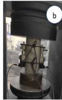
Testing setup for stress strain curve (a) View-1 (b) View-2
