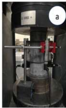
Testing setup for stress strain curve (a) View-1 (b) View-2
