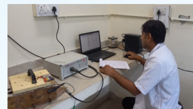
Corrosion rate measurement
