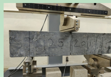
Testing of notched beam in progress for the study of fracture behaviour of High Strength Concrete
