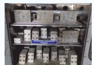
Accelerated Carbonation Induced Corrosion Study
