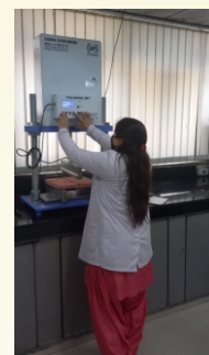
Net Transverse strength of Cement concrete tile using Flexure Testing Machine of 10kN
