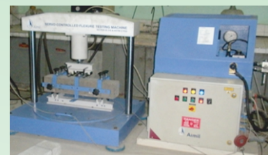
Flexure toughness test on Steel Fibre Reinforced Concrete
