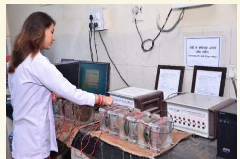
Rapid Chloride Penetrability Test for concrete Samples to study the chloride ions penetrability.
