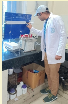
Initial surface absorption test (ISAT) apparatus to evaluate the rate of water absorption by concrete samples
