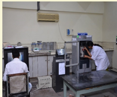
Modulus of Elasticity and Poisson's ratio determination through high precision servo controlled Compression Testing Machine-3000kN
