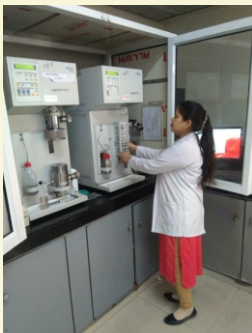
Mercury Intrusion Porosimeter test is used to study the pore size distribution and porosity of aggregate, concrete and mortar.
