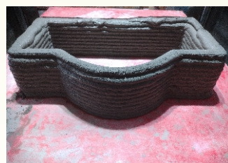
3D Printed Concrete object manufactured using indigenous developed 3D customized printer
