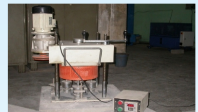
Abrasion Resistance test for Concrete
