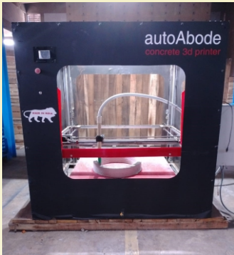
Lab scale 3D concrete printer
