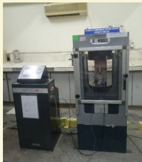
Test for Stress Strain Characteristics in progress for High Strength Concrete
