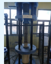
Creep testing in loaded condition
