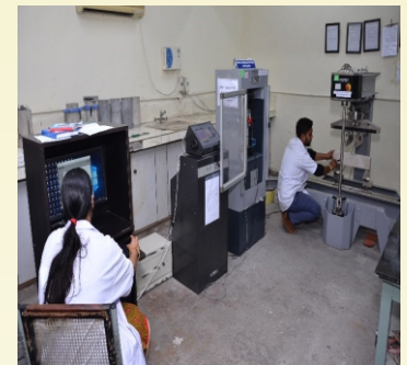
Strain Controlled Flexural Testing Machine-300kN for determination of flexural toughness of fiber reinforced concrete and crack mouth opening gauge for measurement and control of crack width in concrete samples
