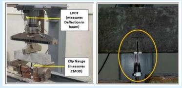
Experimental setup for evaluation of fracture parameters
