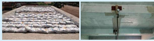
Load testing with sand-filled bags in progress on the RGC slab structure
